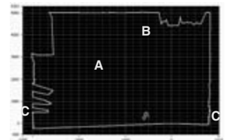
A Near detection field B Far detection field C Current measurement values
