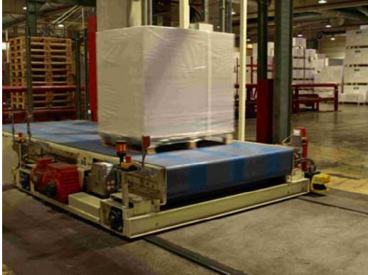
Figure 1. Side-tracking skates are equipped with a Safety Laser Scanner in both directions.
