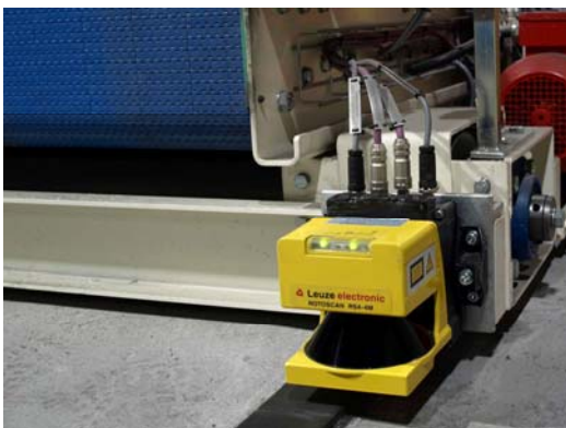
Figure 2. With the help of the PROFIBUS interface, the ROTOSCAN RS4-4M Safety Laser Scanners can quickly be integrated into the safety network.
