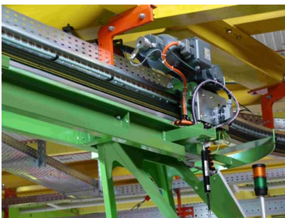
Figure 3 a/b. The CaddyPick® telpher-line vehicles are positioned using the barcode positioning system. The code tape in the guide rail is scanned by the reader in the suspended carriage.
