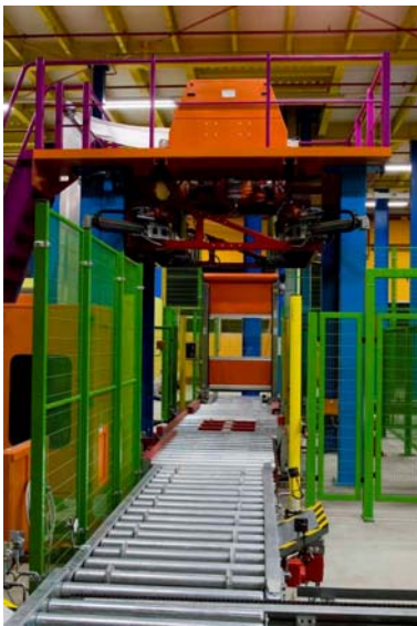
Figure 1. Roller conveyor safeguarding with muting with the COMPACT plus Multiple Light Beam Safety Devices.
