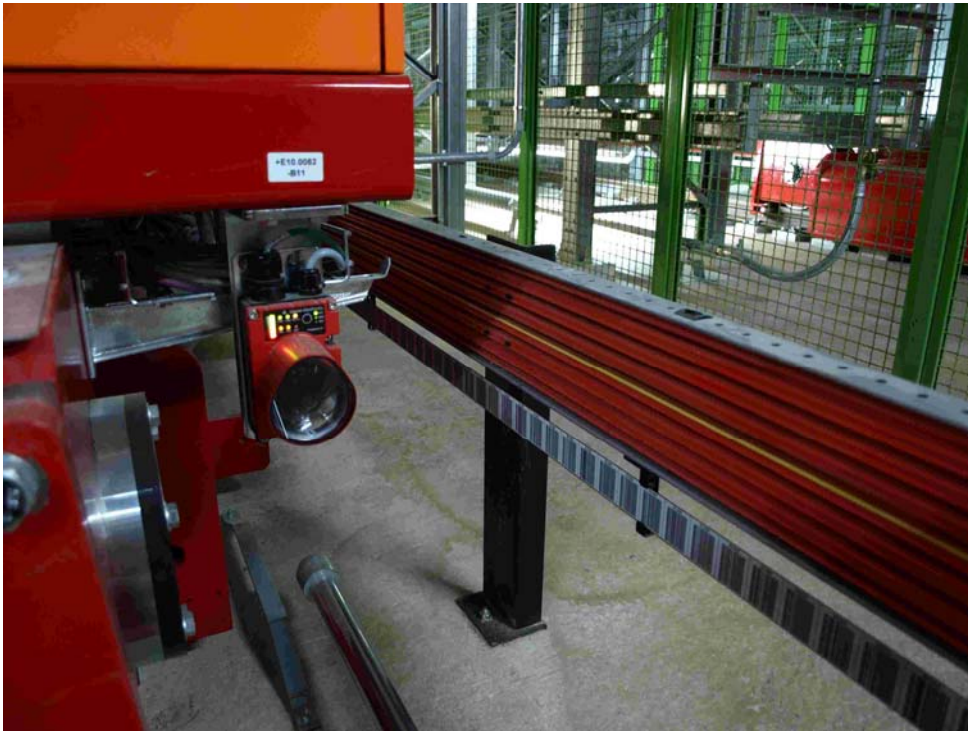
Figure 4. The high-bay storage device is positioned using barcode technology; the position data is transmitted by means of Data Transmission Light Beam Devices.
