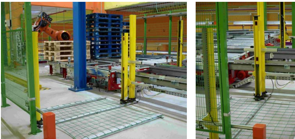
Figure 5 a/b. The muting function of the COMPACT plus Multiple Light Beam Safety Devices ensures permanent personnel protection without interfering with the flow of goods.
