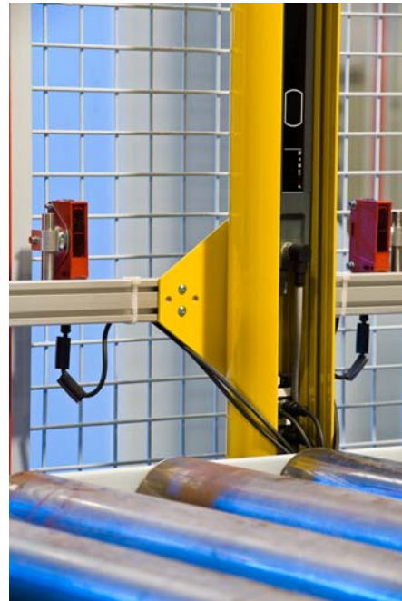
Figure 3. Detailed view of the UDC device column with muting transceiver (in the column) and mounted MMS Muting Mounting System, including prewired muting sensors
