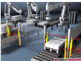
Access guarding with MLD Multiple Light Beam Safety Devices in an application with partial Muting
