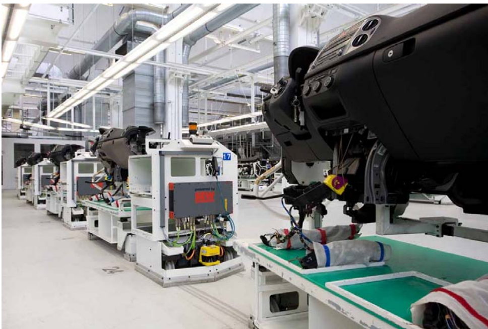
Figure 1. Autonomous operation: Cockpit assembly on Automatic Guided Vehicles (AGV)-a distance of 80 cm between the vehicles was required.
