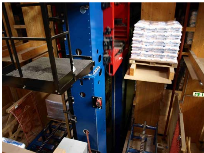
Figure 4. DDLS 200 optical data transmission systems on high-bay storage devices facilitate contact- and wear-free optical communication.
