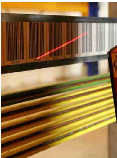
Figure 3. The read head of the BPS 34 always reads multiple codes on the code tape simultaneously (source: LTW Intralogistics GmbH)
