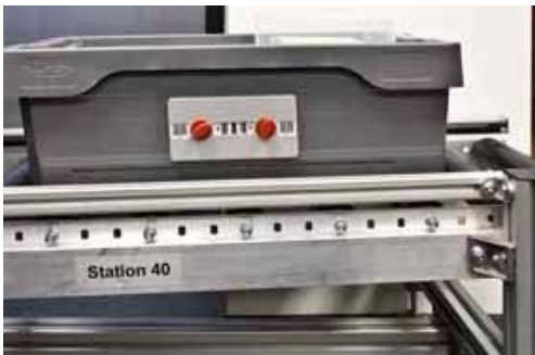
Figure 7. The presetting on the container can be made with either slider coding bars or, as shown here, with rotary coding discs. With the latter variant, the worker can easily and quickly set the destination for the container transport with a turning motion.
