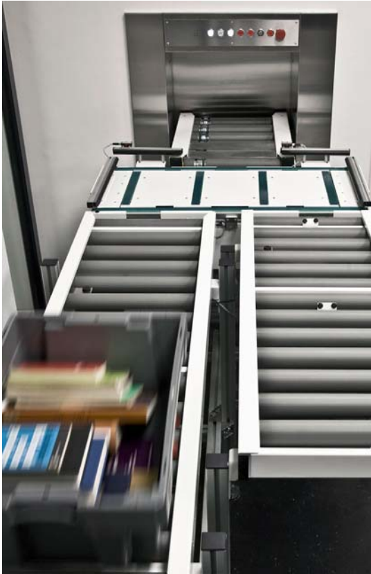
Figure 4. The container moves quickly towards the vertical conveyor – a fully automatic lift that functions similar to a paternoster to transport books between the individual levels of a building.
