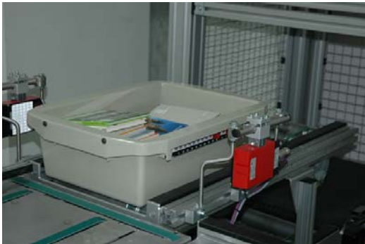
Figure 2. Transport solutions with Leuze electronic coding bars for the barcode readers provide greater efficiency in handling the book quantities encountered in large libraries.
