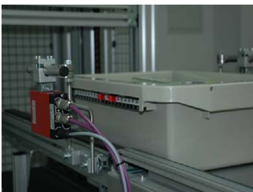
Figure 8. Unlike rotary coding discs, containers with side-mounted coding bars can be optimally stacked inside of one another, i.e. they can be nested and stored in a space-saving manner.
