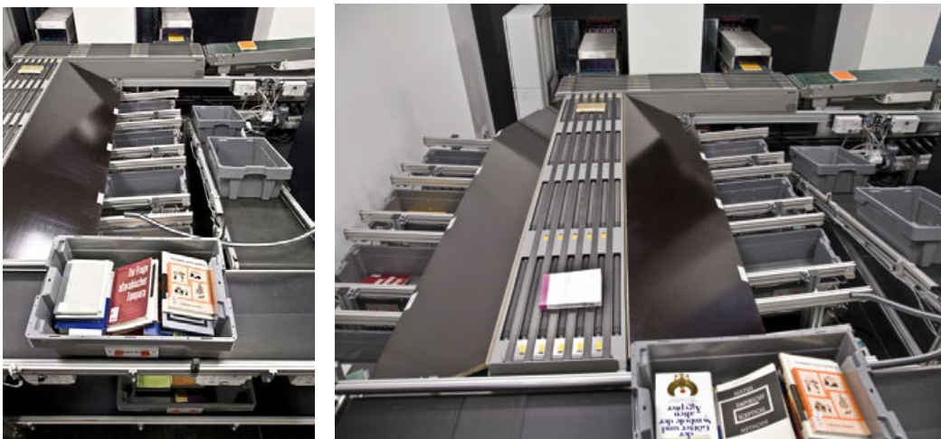
Figure 1 a, b. Swisslog-Telediff light conveyor systems for the automated transport of books in libraries
