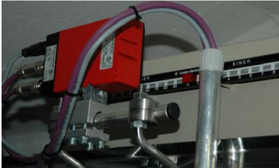
Figure 9. The coding bars are set by sliding red positioning elements so that they cover certain barcodes for the readers.
