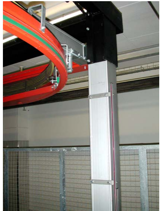
Installation position of the VARIO light grid for the detection of 7 µm thick foil
