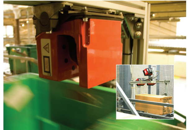
ABOVE: Leuze electronic ROD 4 scanners are used to check contents of tote bins
