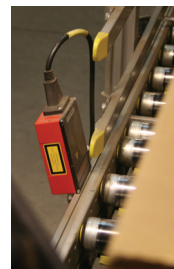
Tray and carton transfer cycles are controlled via strategically positioned BCL 40 barcode readers, tracking cartons by reading the code on the slim carrier tray
