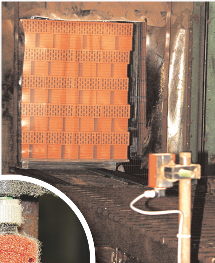
Sensors in the brickworks must continue to operate reliably, even when coated with dust and fluff created by cutting rock wool mats for insulating bricks (left)
