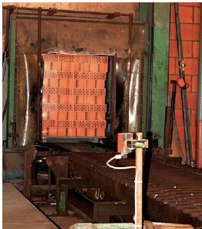
ABOVE: The entire production sequence at Zeller is controlled electronically. The signals necessary for this purpose are supplied by sensors from Leuze electronic
