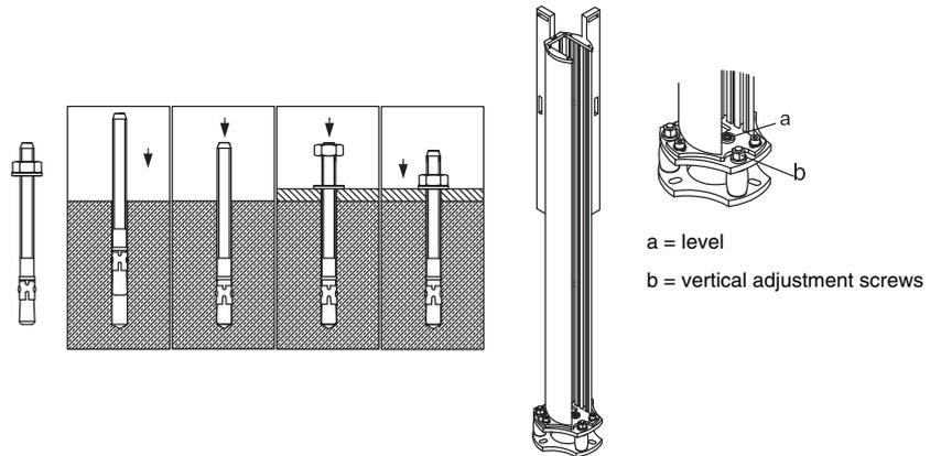
1. The devices come already mounted in the device column UDC. The installation height can be adjusted by loosening the Allen screws of the device brackets in the column.
