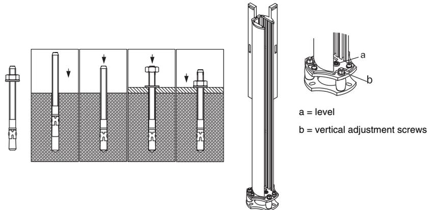
1. The devices come already mounted in the device column UDC. The installation height can be adjusted by loosening the Allen screws of the device brackets in the column.
